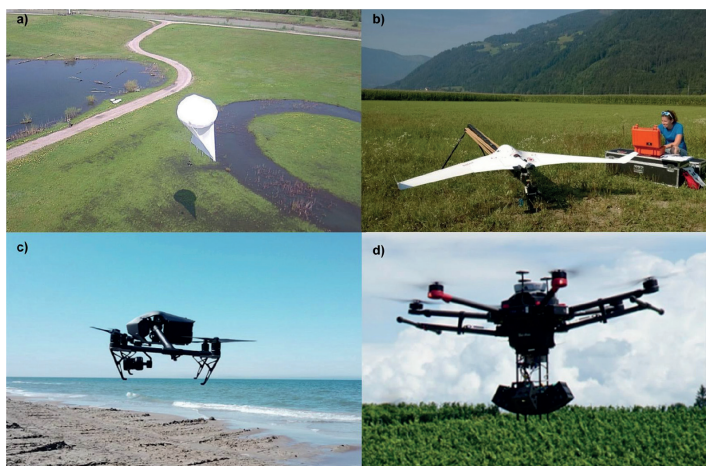
Fig. 1. Different platforms and sensors in UAS surveys; a) Lighter-Than-Air Helikite Balloon with Sony A7RII used for renaturation monitoring; b) BRAMOR ppk Fixed-Wing with Micasense Red Edge used for riparian vegetation monitoring; c) DJI Inspire 2 with zennuse x5s RGB camera, used for shallow water vegetation and beach cast monitoring (Palanga, Lithuania), and d) Leica Aibot AX 20 with multidirectional sensor prototype (5 Sony ILCE-QX1 RGB sensors for capturing NADIR and 4 oblique images). (For interpretation of the references to colour in this figure legend, the reader is referred to the web version of this article.)
